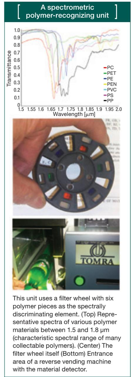
[ Polymer-recognizing spectrometer based on a diffractive optical element ]
